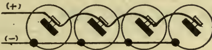
FIG. 182.—Diagram of a multiple or parallel connection. When connected in this manner the voltage of the battery is the same as that of a single cell, but the amperage of the battery is equal to the amperage of a single cell multiplied by the number of cells.
